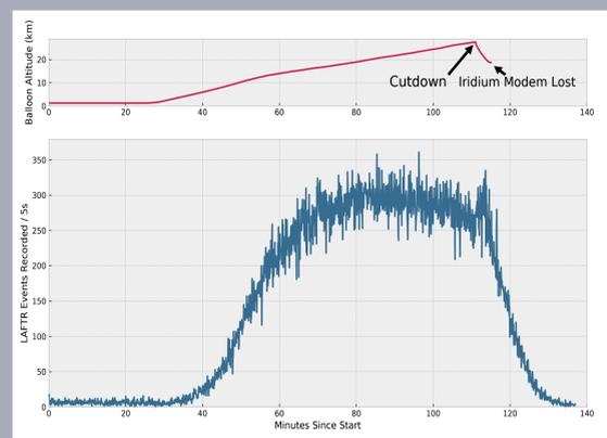
Count rate data from November, 12th test flight. Also shown is the balloon's altitude. Shortly after cutdown, the Iridium modem (onboard an accompanying payload) was abruptly lost. As such, no altitude data is available for the remainder of the flight.
